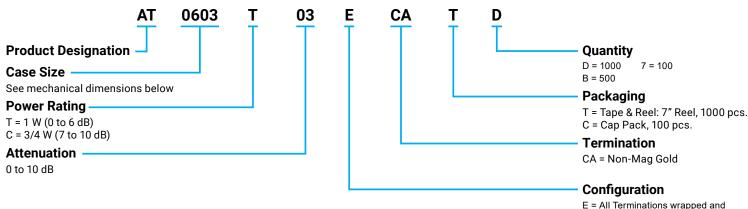
The above part number refers to an AT 0603 Case Size with an attenuation of 3dB, 1W Power Rating, wrapped and patterned ground plane configuration with Solderable Gold Termination and tape and reel packaging, 1000 pcs.
