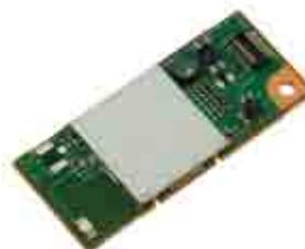
WLAN Original Antenna & Board to Board Connector
