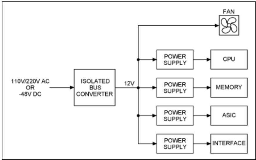
Figure 1. A typical power-supply arrangement.
