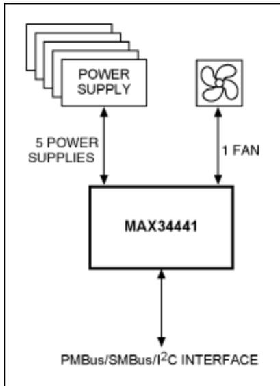
Figure 5. A pizza-box system design using the MAX34441.
