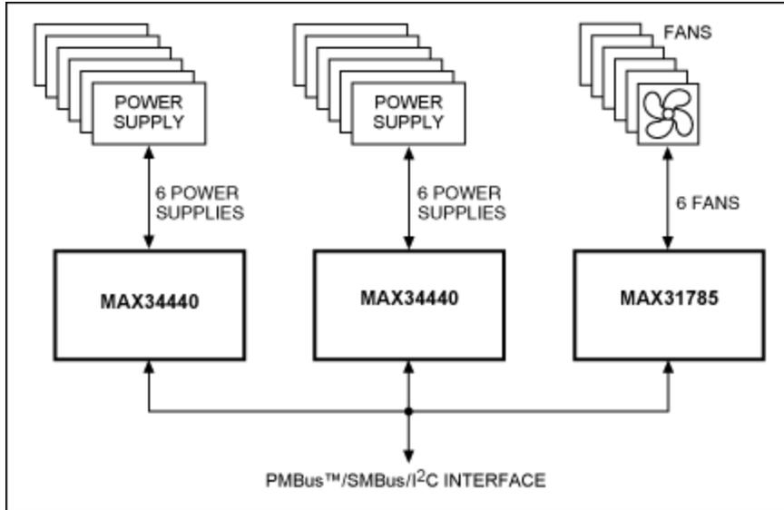
Figure 4. A big-box system design uses the MAX34440 and MAX31785.
