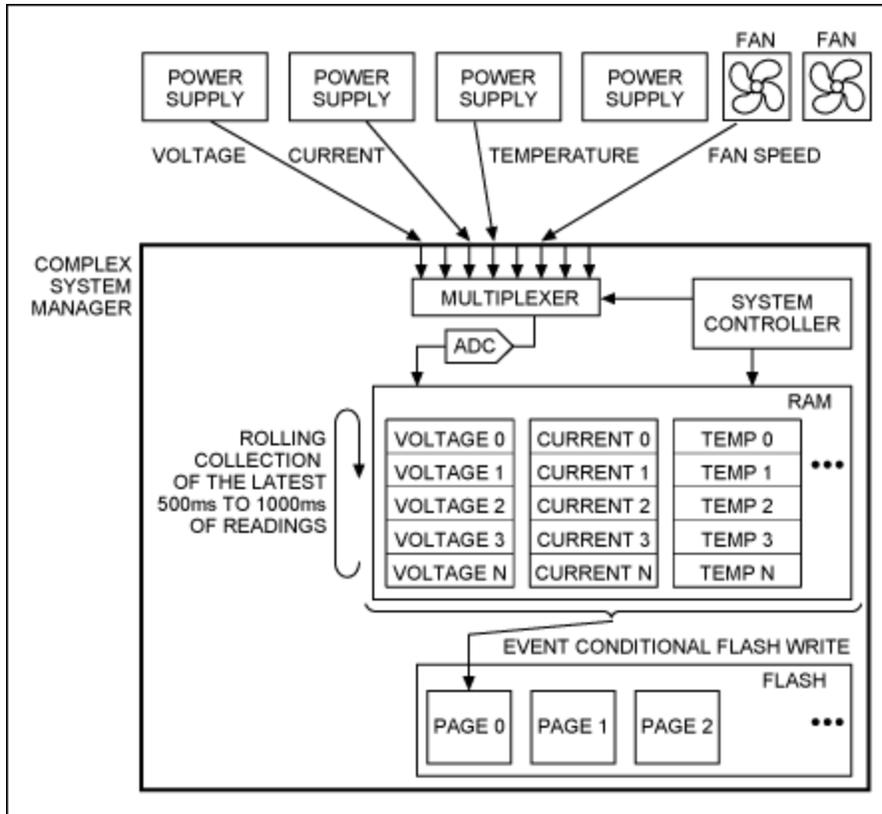
Figure 2. Functional diagram of a nonvolatile fault-logging system for a number of power supplies and fans.
