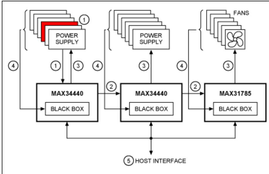
Figure 3. Black-box fault logging scenario.
