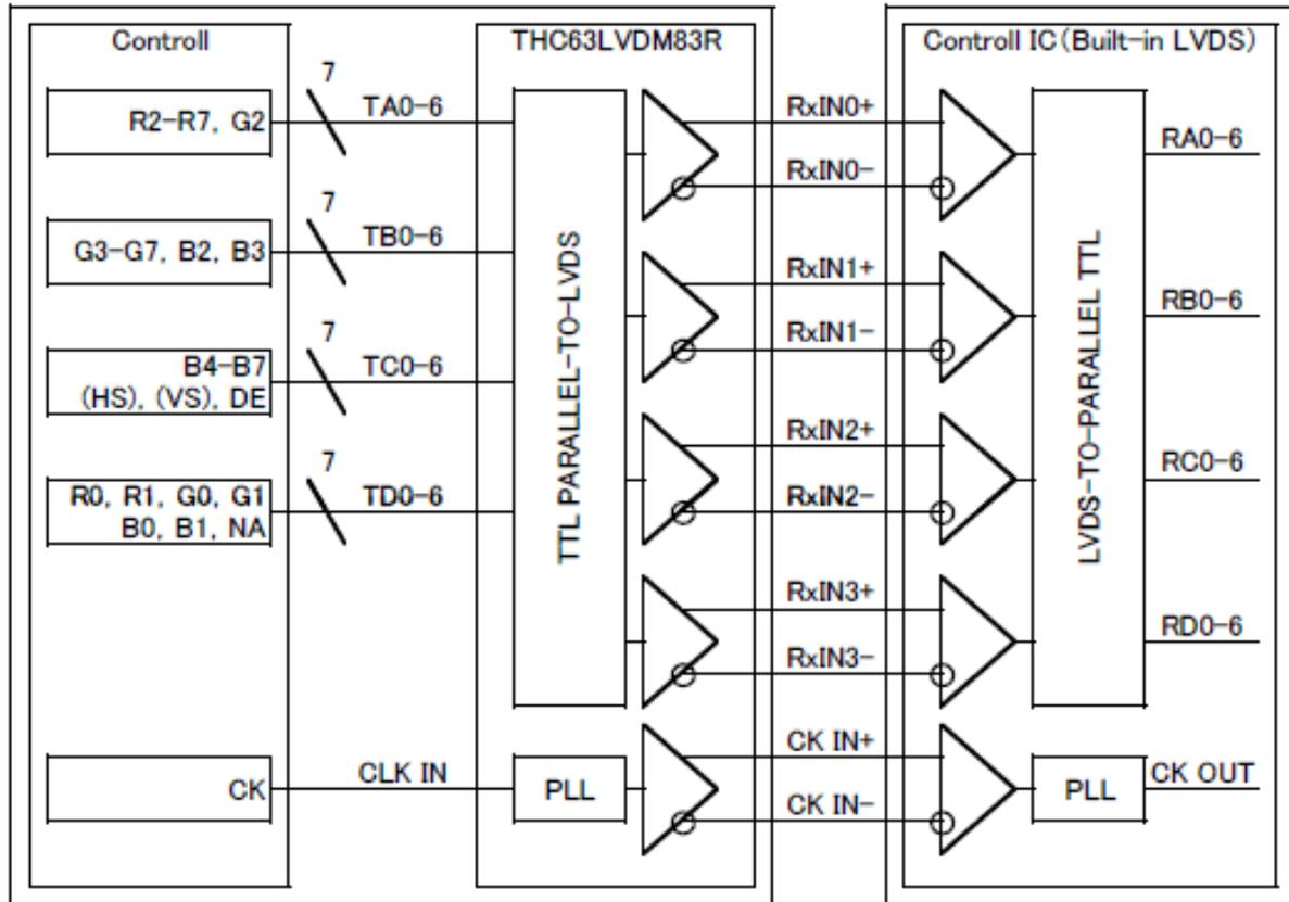
7-4. Data mapping (6bit input / 6bit mode)
