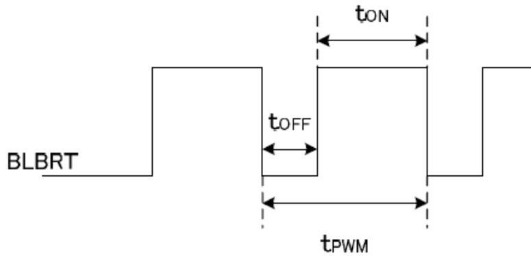
$t_{ON}, t_{OFF} = 50 \mu s$ .
