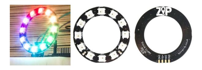
Add light to your latest project with the Kitronik ZIP Circle. Each Circle has 12 individually addressable RGB LEDs which can be coded with the PXT Editor.
