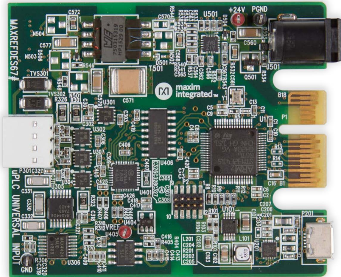
Figure 9. MAXREFDES67# System Board.
