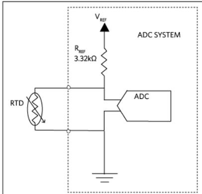
Figure 2. 2-wire constant voltage excitation configuration.
