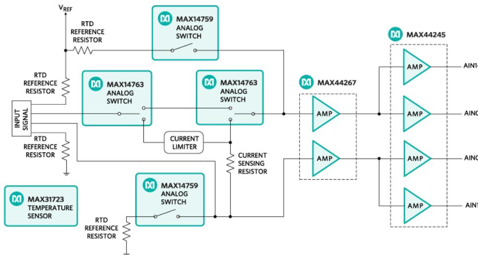
Figure 11. MAXREFDES67# Input Circuits Block Diagram.
