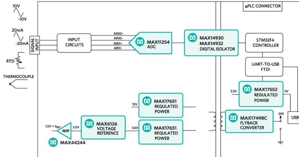
Figure 10. MAXREFDES67# Reference Design Block Diagram.
