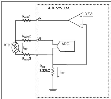
Figure 3. 3-wire constant current excitation configuration.
