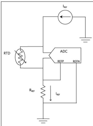
Figure 7. Current excitation configuration for ratiometric measurement.
