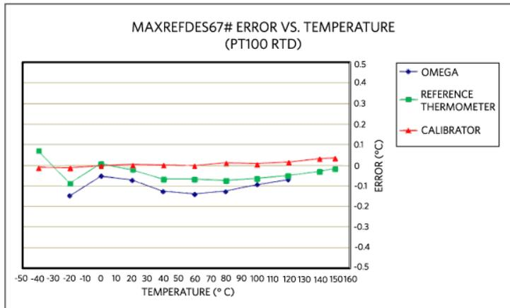
Figure 12. MAXREFDES67# error vs temperature, using an Omega P-M-1/10-1/4-6-0-G-3, 4-wire RTD calibrated at 20°C.
