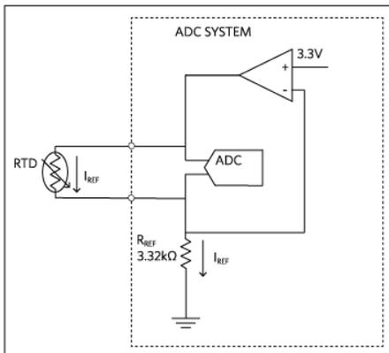
Figure 1. 2-wire constant current excitation configuration.
