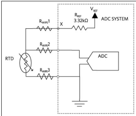
Figure 4. 3-wire constant voltage excitation configuration.
