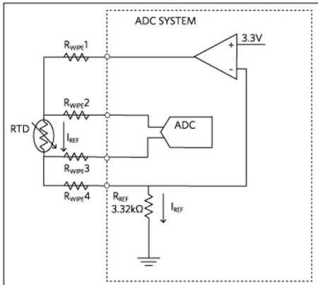
Figure 5. 4-wire constant current excitation configuration.
