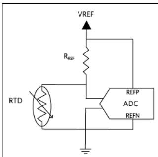
Figure 8. Voltage excitation configuration for ratiometric measurement.
