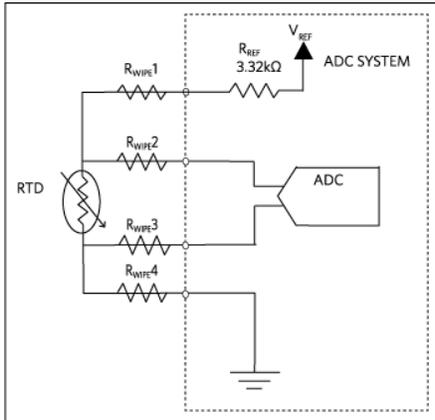
Figure 6. 4-wire constant voltage excitation configuration.
