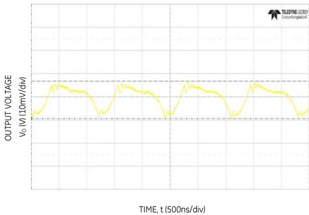
Figure 27. Typical output ripple and noise (C<sub>O</sub>=2x47µF ceramic, V<sub>IN</sub> = 12V, I<sub>o</sub> = I<sub>o,max</sub>.)
