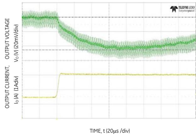
Figure 28. Transient Response to Dynamic Load Change from 50% to 100% at 12V<sub>in</sub>, C<sub>out</sub>=2x47µF+1x330µF, C<sub>Tune</sub>=6800pF, R<sub>Tune</sub>=300
