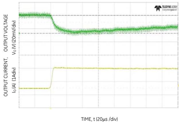
Figure 16. Transient Response to Dynamic Load Change from 50% to 100% at 12Vin,  $C_{out}=4 \times 47 \mu F + 1 \times 330 \mu F$ ,  $C_{Tune}=15nF$ ,  $R_{Tune}=300$
