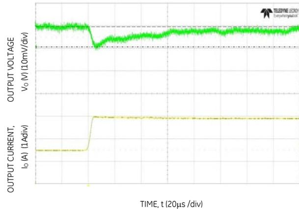
Figure 4. Transient Response to Dynamic Load Change from 50% to 100% at 12Vin, C<sub>out</sub>=8x47uF+1x330uF, CTune=5.6nF, RTune=300Ω
