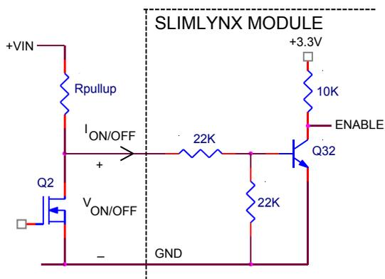
Figure 39. Circuit configuration for using negative On/Off logic.
