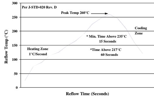
Figure 49. Recommended linear reflow profile using Sn/Ag/Cu solder.
