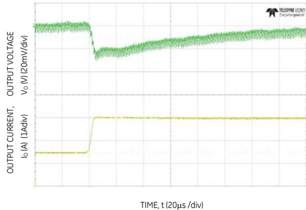
Figure 34. Transient Response to Dynamic Load Change from 50% to 100% at 12Vin, Cout=2x47µF+1x330µF, CTune=2700pF, RTune=300Ω
