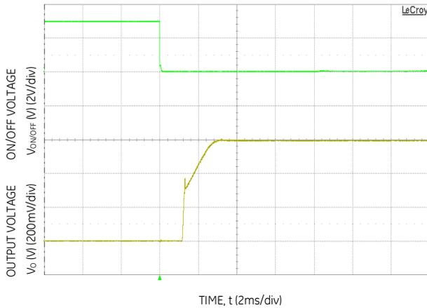
Figure 5. Typical Start-up Using On/Off Voltage (I<sub>o</sub> = I<sub>o,max</sub>).
