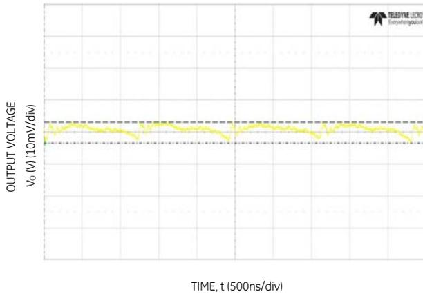
Figure 3. Typical output ripple and noise (C<sub>o</sub>=2x47μF ceramic, V<sub>IN</sub> = 12V, I<sub>o</sub> = I<sub>o,max</sub>).
