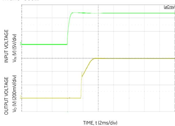
Figure 6. Typical Start-up Using Input Voltage (V<sub>IN</sub> = 12V, I<sub>o</sub> = I<sub>o,max</sub>).
