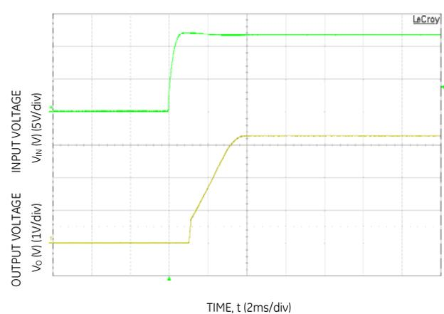
Figure 30. Typical Start-up Using Input Voltage (V<sub>IN</sub> = 12V, I<sub>o</sub> = I<sub>o,max</sub>).
