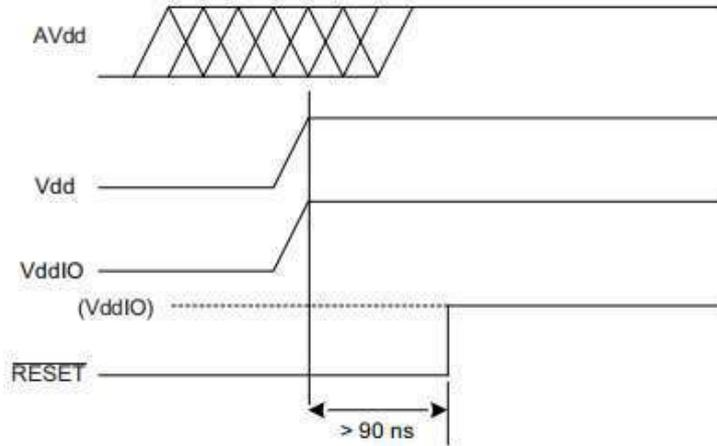
Note: When using external  $\overline{\text{RESET}}$  at power-up, VddIO must not be enabled after Vdd
