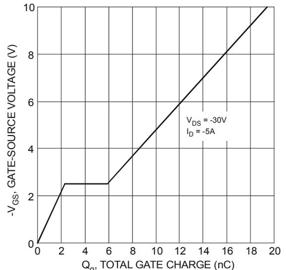
Figure 22 Gate-Charge Characteristics
