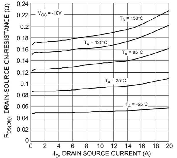
Figure 16 Typical On-Resistance vs. Drain Current and Temperature
