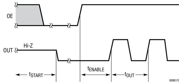
Figure 9. Start-Up Timing Diagram (OE = 0, N<sub>DIV</sub> = Any, Hi-Z = 0)
