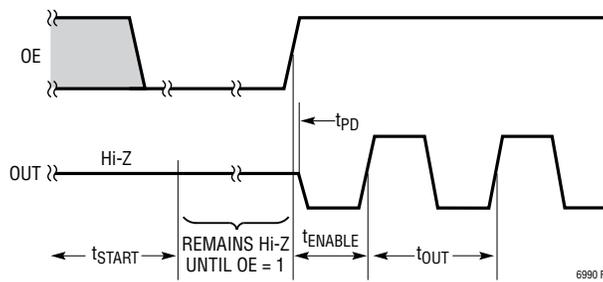
Figure 10. Start-Up Timing Diagram (OE = 0, N<sub>DIV</sub> = Any, Hi-Z = 1)
