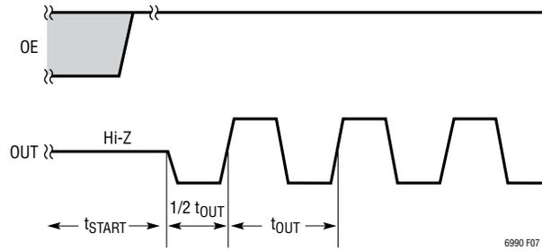
Figure 7. Start-Up Timing Diagram (OE = 1, N<sub>DIV</sub> = 1 or 2, Hi-Z = 0 or 1)
