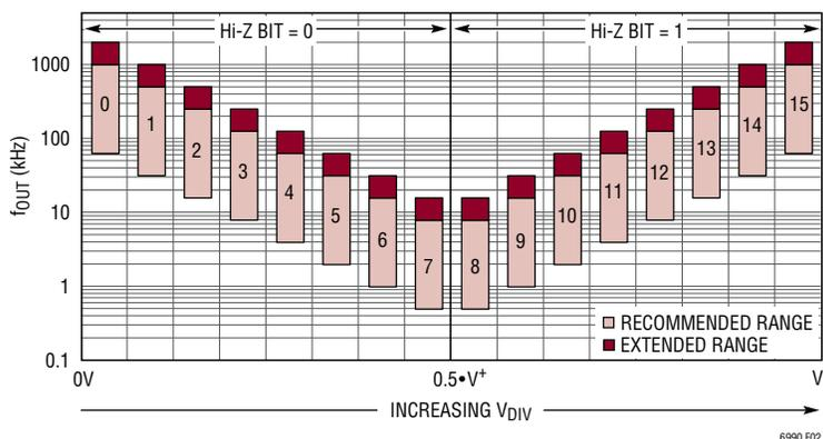
**Figure 2. Frequency Range and Hi-Z Bit vs DIVCODE**
