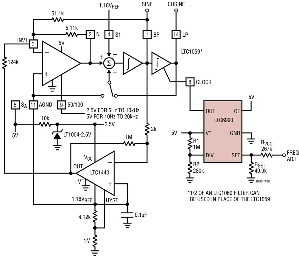
**Temperature to Frequency Converter. 3% Linearity from -20°C (f<sub>OUT</sub> ≈ 20kHz) to 75°C (f<sub>OUT</sub> ≈ 25kHz)**
