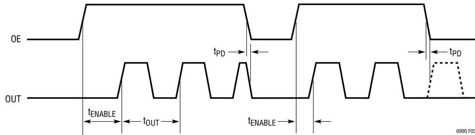
**Figure 3. OE Timing Diagram (Hi-Z = 0)**
