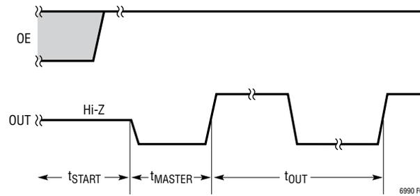
Figure 8. Start-Up Timing Diagram (OE = 1, N<sub>DIV</sub> ≥ 4, Hi-Z = 0 or 1)
