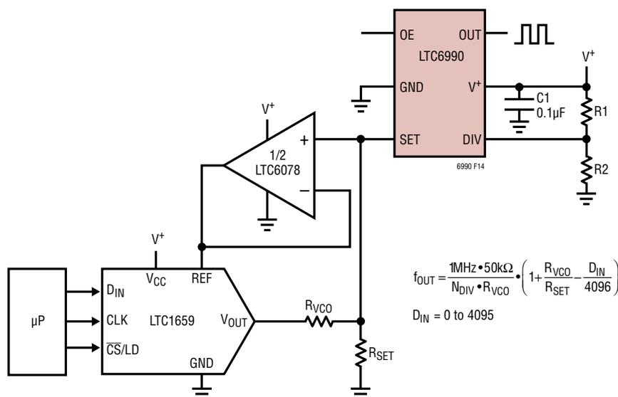
Figure 14. Digitally Controlled Oscillator with  $V_{SET}$  Variation Eliminated
