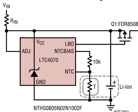
**NTC Overtemperature Battery Float Voltage Qualifying**
