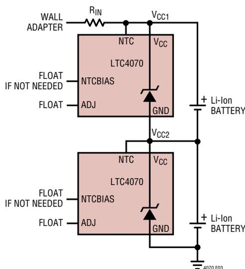
Figure 3. 2-Cell Battery Charger
