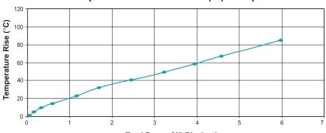
**Total Power (W) Dissipation** Total Power Dissipation (W) = .001 \* (DCRprimary \* IRMs primary² + DCRsecondary \* IRMs secondary²) + Core Loss (W)
