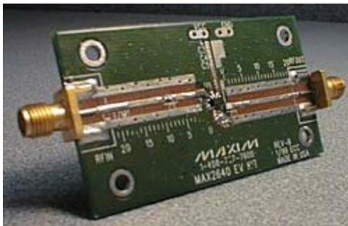
*Objective: To tune the MAX2640 for operation at 345MHz for wireless security-system transmission.*
