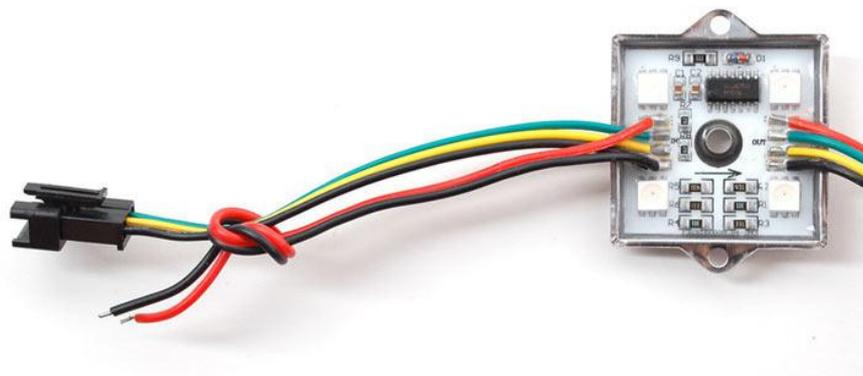
Wiring is pretty easy since there are only 4 wires. The only important thing is that you should not try to power the LED strand from the Arduino's 5V line — these LEDs require a dedicated 12V source separate from the microcontroller.
