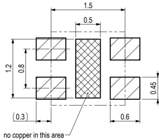
**Figure 12:** Recommended land pattern (in mm). Details can vary and depend on used PCBs and solder processes. There shall be no copper under the sensor other than at the pin pads.
