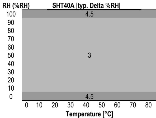
**Figure 4:** Typical RH accuracy tolerance over humidity and temperature for SHT40A.
