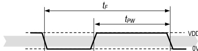
**Figure 9** PWM signal: The base frequency of  $1/t_F$  remains constant, whereas  $t_{PW}$  is variable. The physical signal of temperature and humidity is provided as  $t_{PW}/t_F$  on the respective pins.
