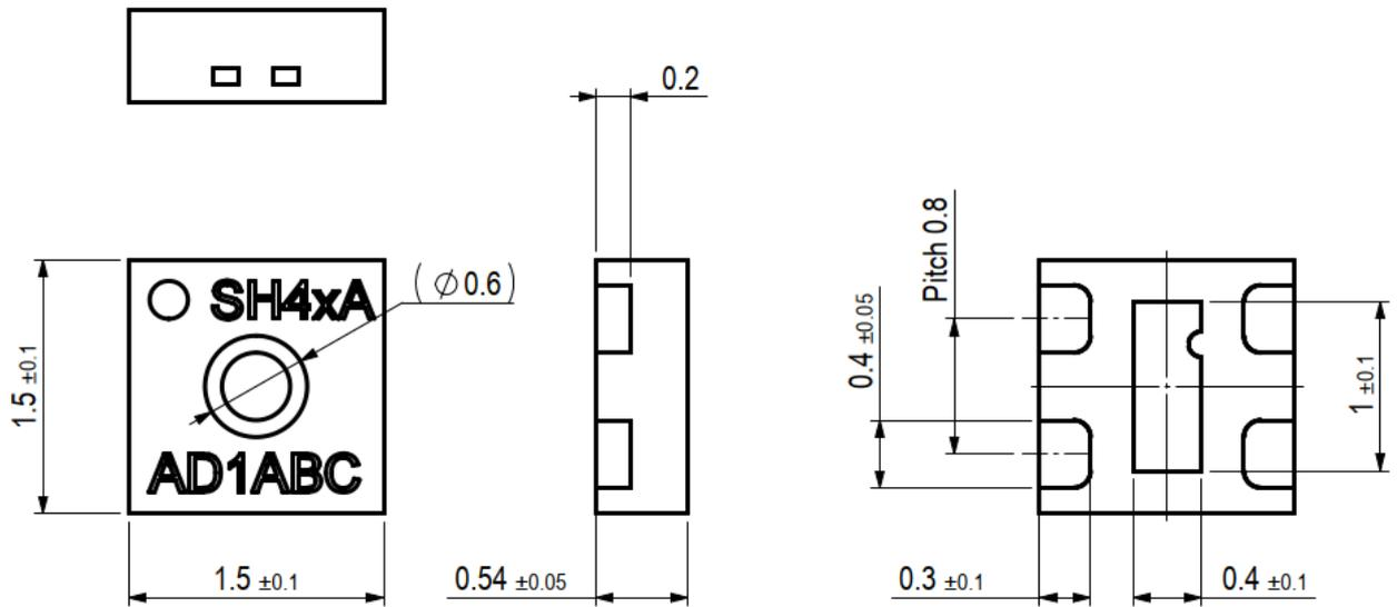
**Figure 10** Dimensional drawing of SHT4xA including package tolerances (units mm).
