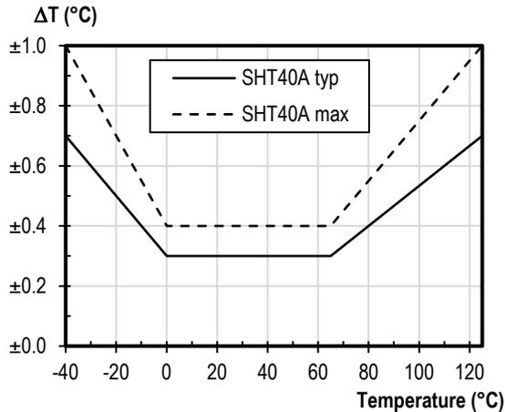
**Figure 6:** SHT40A typical and maximal temperature accuracy.
