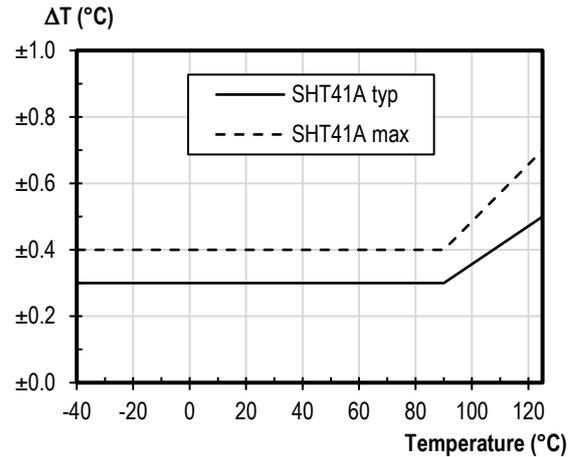
**Figure 7:** SHT41A typical and maximal temperature accuracy.
