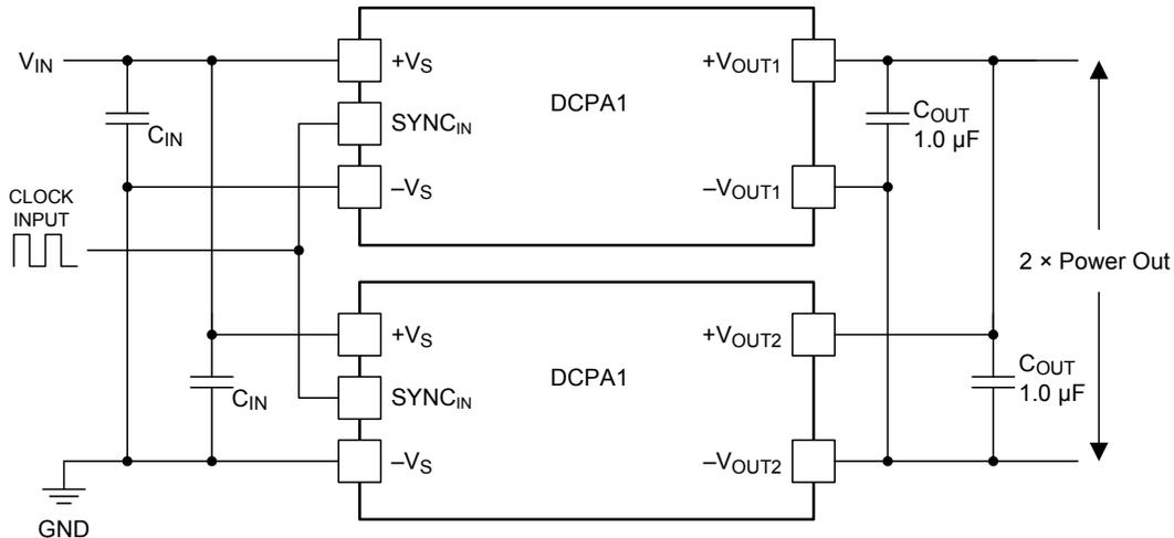
Figure 36. Multiple DCPA1 Devices Connected in Parallel
