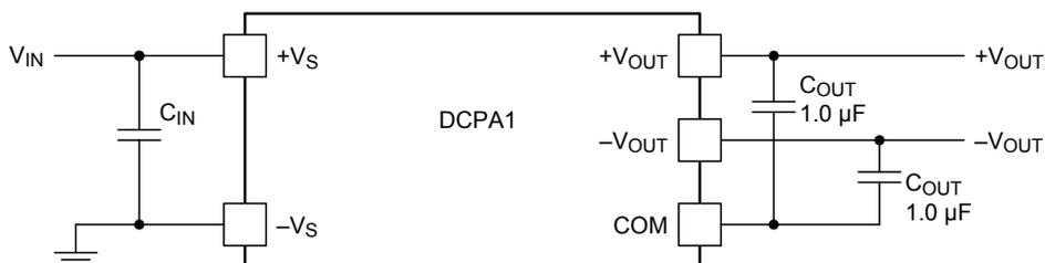
Figure 35. Dual Output Devices Connected in Series
