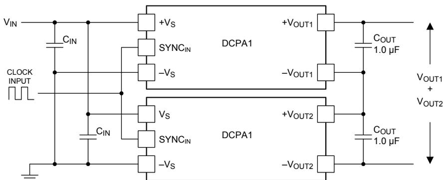
Figure 34. Multiple DCPA1 Devices Connected in Series
