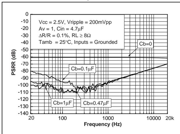
The two following graphs show typical applications of the TS4994 with a random selection of four  $\Delta R/R$  values with a 0.1% tolerance.
