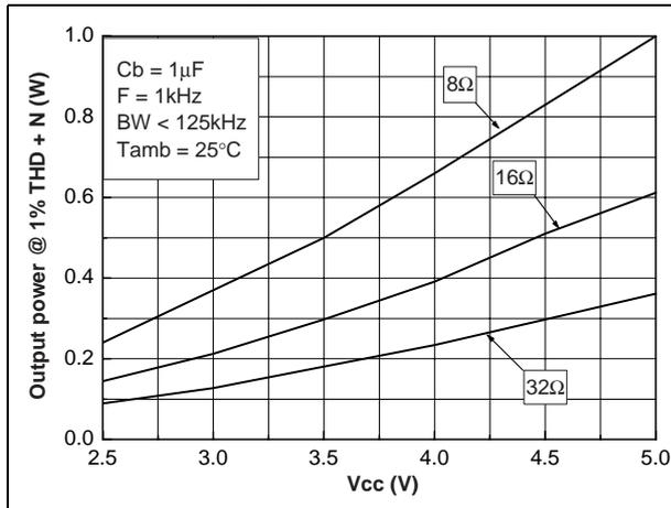
Figure 12. Output power vs. power supply voltage
