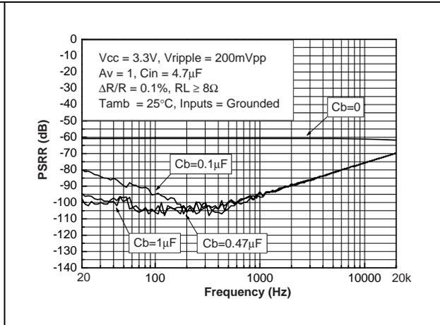
**Figure 72. PSRR vs. frequency (worst case conditions)**
