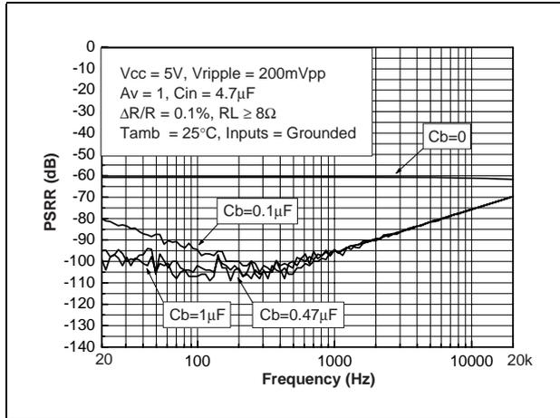
**Figure 71. PSRR vs. frequency (worst case conditions)**
