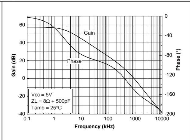
Figure 17. Open loop gain vs. frequency
