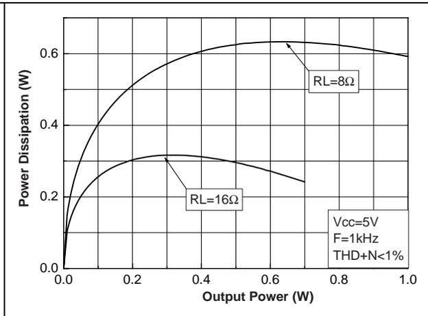
Figure 9. Power dissipation vs. output power
