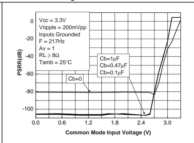
Figure 33. PSRR vs. common mode input voltage
