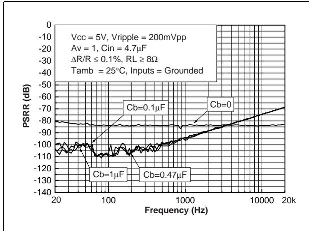
**Figure 74. PSRR vs. frequency with random choice condition**
