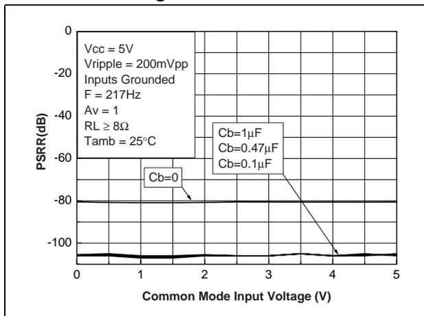
Figure 32. PSRR vs. common mode input voltage
