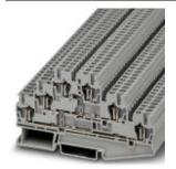
Multi-level terminal block, with diode1N4007, Connection method: Spring-cage connection, Cross section: 0.08 mm² - 4 mm², AWG: 28 - 12, Width: 5.2 mm, Color: gray, Mounting type: NS 35/7,5, NS 35/15
