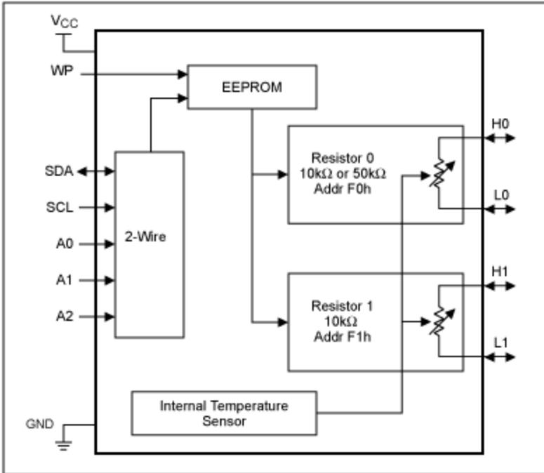
Figure 1. Block diagram.
