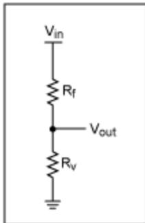
Figure 6. Voltage divider.
