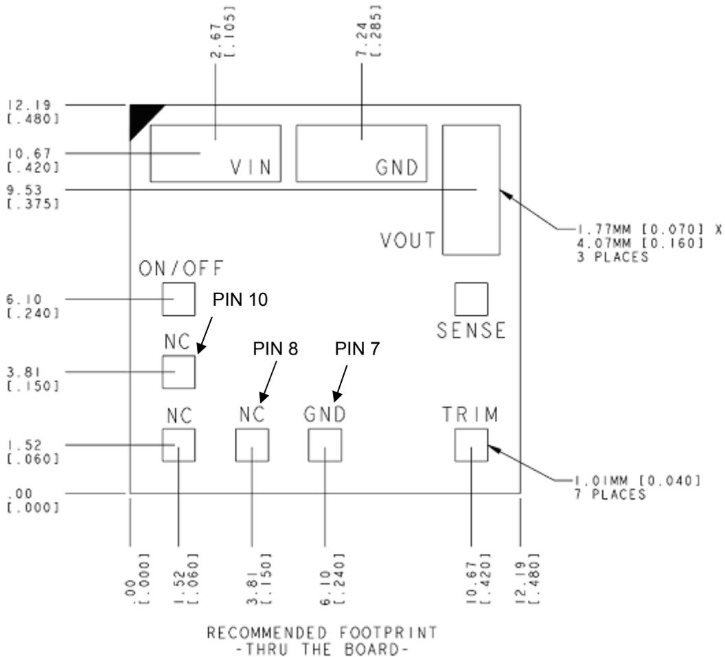
Dimensions are in millimeters and (inches).
