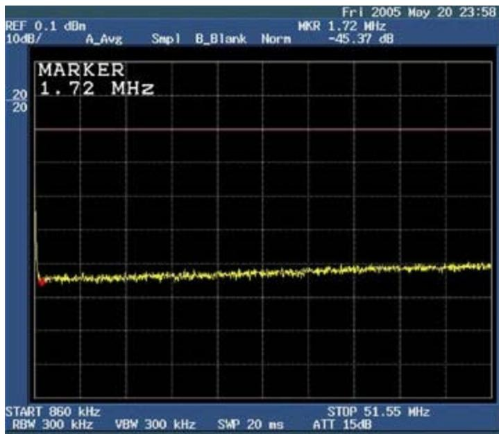
Figure 2. Return loss of  $75\Omega$  test load.
