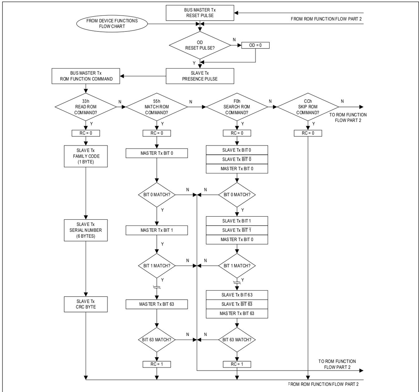
Figure 3. 1-Wire ROM Function Flow Part 1
