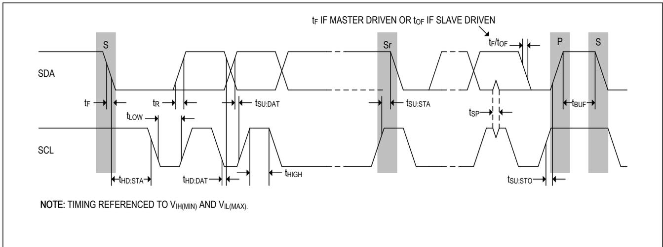
Figure 10. I<sup>2</sup>C Timing Diagram
