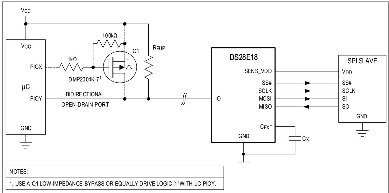
Figure 14. DS28E18 Configured as an SPI Master
