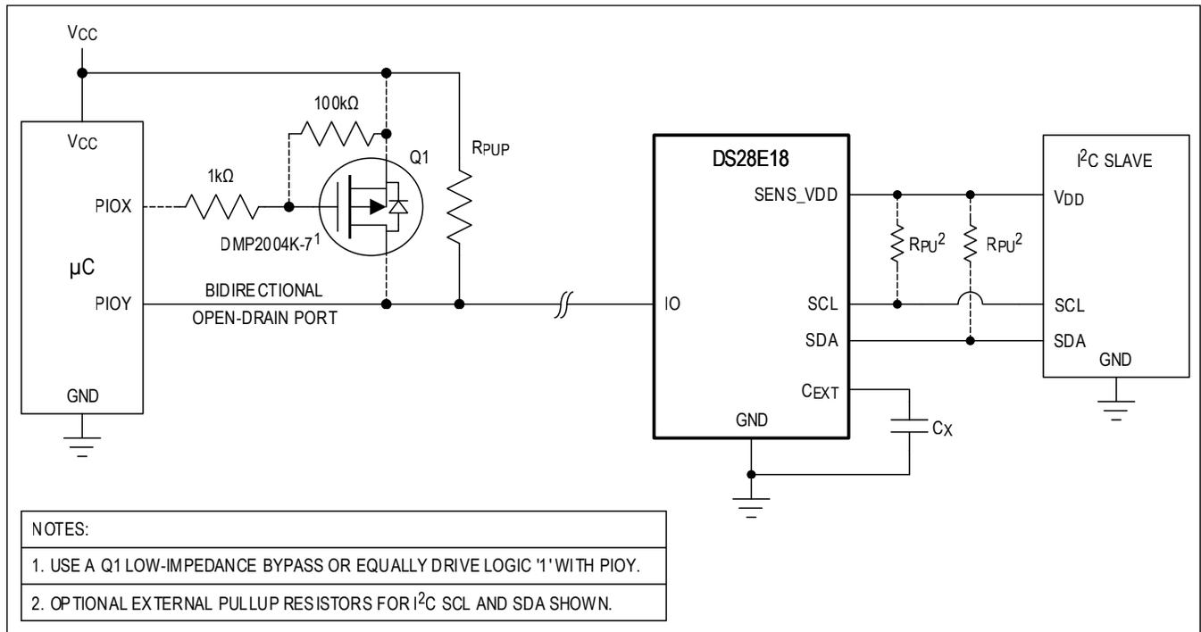
Figure 13. DS28E18 Configured as an I<sup>2</sup>C Master
