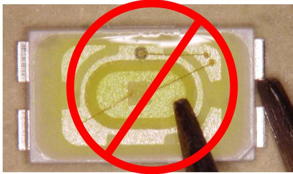
(2) In general, LEDs should only be handled from the side. This also applies to LEDs without a silicone sealant, since the surface can also become scratched.
