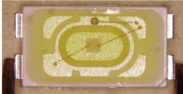
(3) When populating boards in SMT production, there are basically no restrictions regarding the form of the pick and place nozzle, except that mechanical pressure on the surface of the resin must be prevented. This is assured by choosing a pick and place nozzle which is larger than the LED's reflector area.
