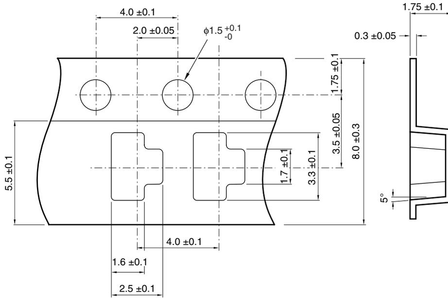
**Fig. 6 Reel Shape and Dimension**
