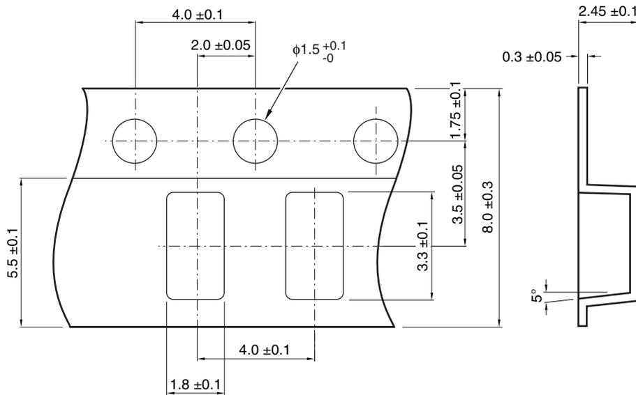
Fig. 9 Reel Shape and Dimension
