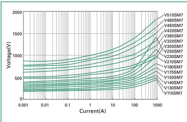
NOTE: If pulse ratings are exceeded, a shift of  $V_{N(DC)}$  (at specified current) of more than  $\pm 10\%$  could result. This type of shift, which normally results in a decrease of  $V_{N(DC)}$ , may result in the device not meeting the original published specifications, but it does not prevent the device from continuing to function, and to provide ample protection.
