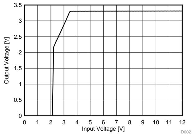
**Figure 1. TLV2217-33 Output Voltage vs Input Voltage**
