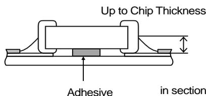
[Standard Conditions for Flow Soldering]
