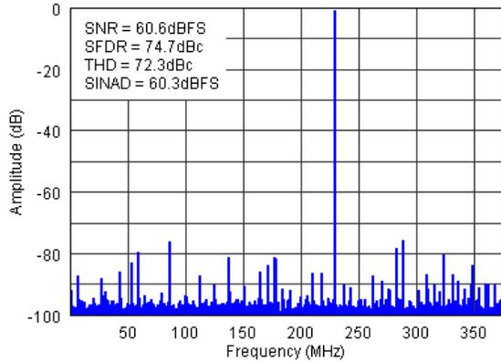
Figure 7-4. FFT for 230-MHz Input Signal (Auto On)
