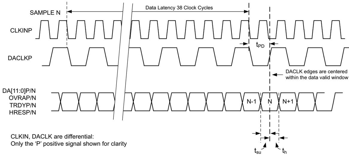
**Figure 7-1. Timing Diagram for 12-Bit DDR Output**
