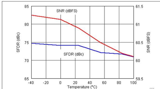
Figure 7-20. Performance Across Temperature (fin = 230 MHz)
