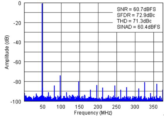
Figure 7-9. FFT for 700-MHz Input Signal (Auto Off)
