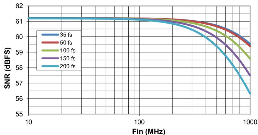
**Figure 8-4. SNR vs. Frequency and External Clock Jitter**
