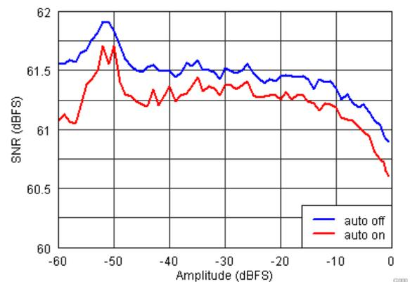
Figure 7-13. SNR vs. Amplitude (fin = 230 MHz)
