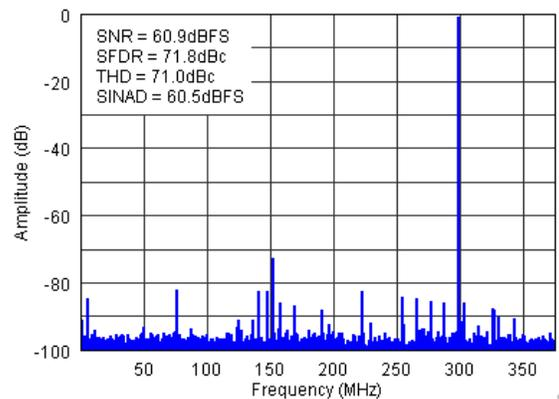
Figure 7-7. FFT for 450-MHz Input Signal (Auto Off)
