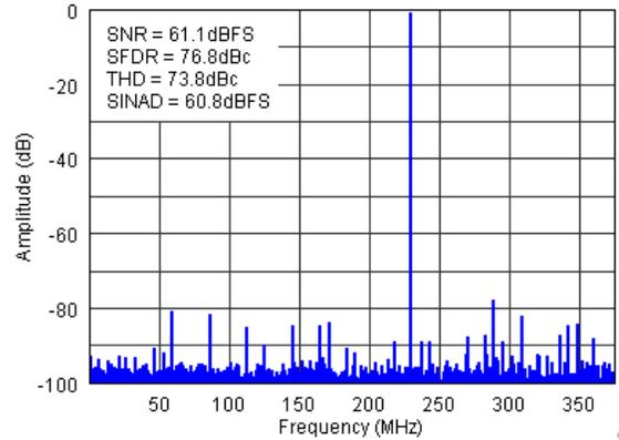
Figure 7-5. FFT for 230-MHz Input Signal (Auto Off)
