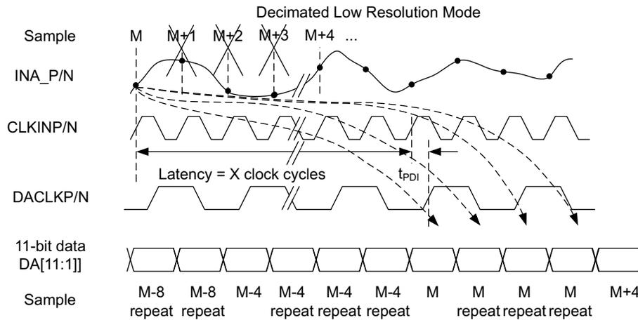
Figure 8-11. Decimated Low-Resolution Output Data Timing Diagram
