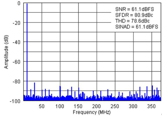
Figure 7-3. FFT for 10-MHz Input Signal (Auto Off)
