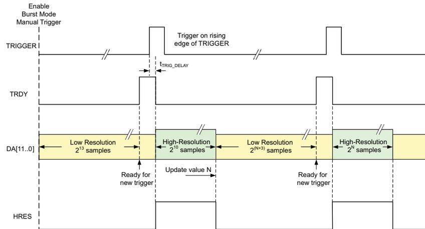
**Figure 8-17. Triggering High Resolution Mode and Lockout Time**
