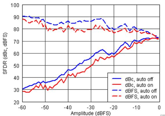
Figure 7-12. SFDR vs. Amplitude (fin = 230 MHz)
