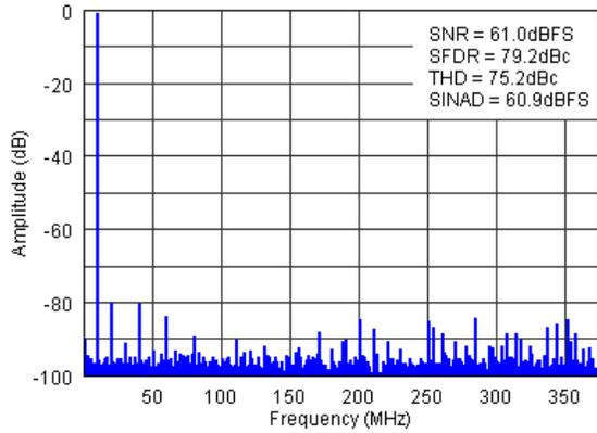
Figure 7-2. FFT for 10-MHz Input Signal (Auto On)
