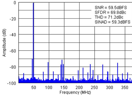
Figure 7-8. FFT for 700-MHz Input Signal (Auto On)
