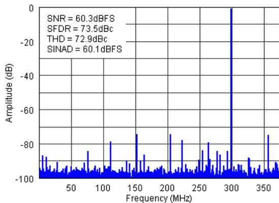
Figure 7-6. FFT for 450-MHz Input Signal (Auto On)
