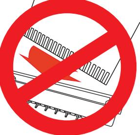
**Do not keep FFC inclined when insertion**
