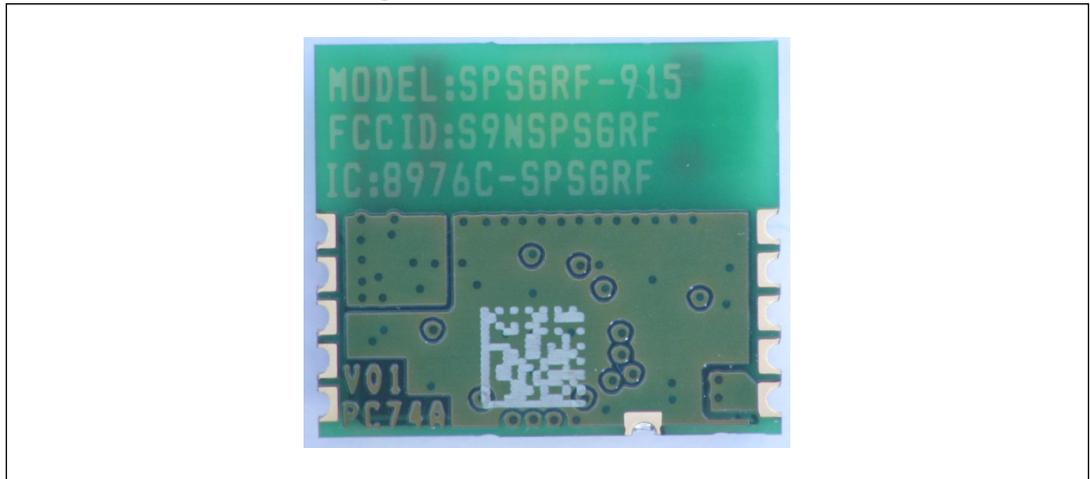
Each module is univocally identified by serial number stored in a 2D laser data matrix marked on the bottom of the module.
