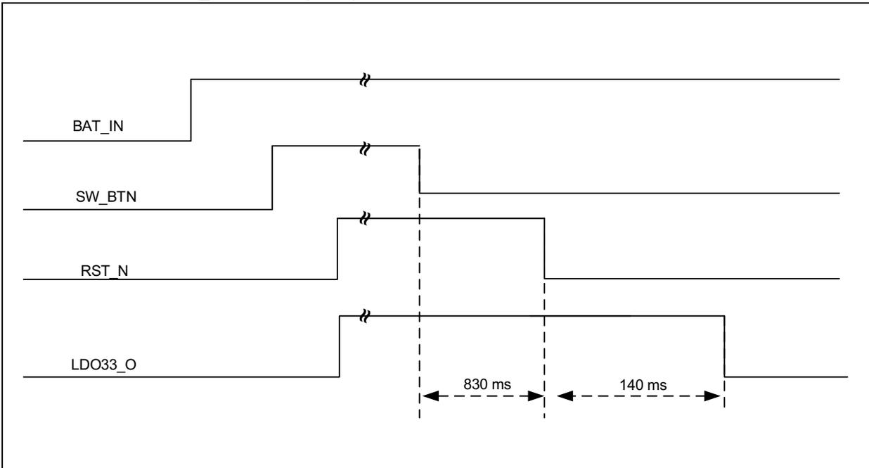
**Note 1:** 830 ms time duration is a typical value measured on iPhone® 6 and this time duration can vary from one smartphone to another.
