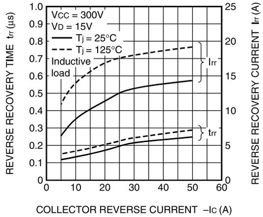
**SWITCHING RECOVERY LOSS CHARACTERISTICS (TYPICAL)**
