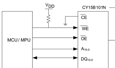
For applications that require the lowest power consumption, the  $\overline{CE}$  signal should be active (LOW) only during memory accesses.
