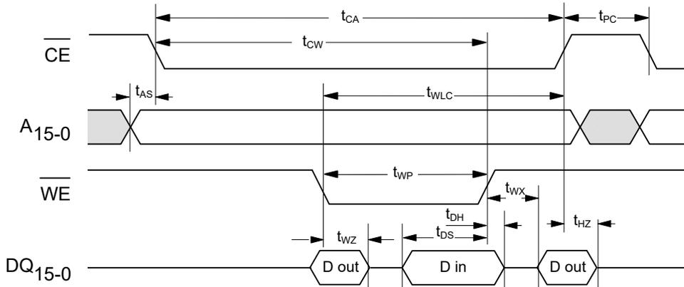
Figure 9. Write Cycle Timing No. 2 ( $\overline{CE}$  Controlled)
