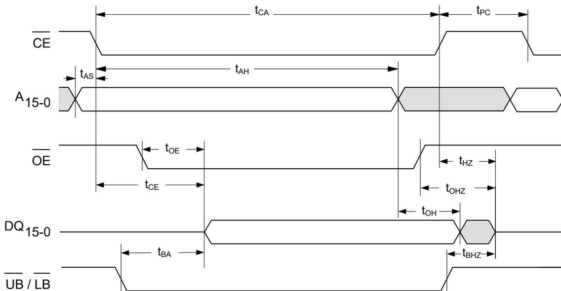
Figure 7. Page Mode Read Cycle Timing <sup>[7]</sup>
