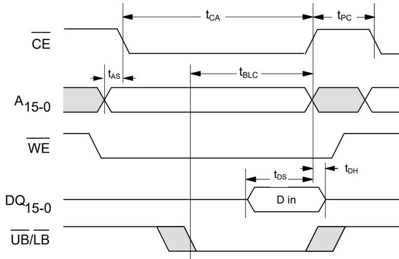
Figure 10. Write Cycle Timing No. 3 ( $\overline{CE}$  LOW) [8]
