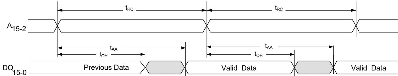
Figure 6. Read Cycle Timing No. 2 ( $\overline{CE}$  Controlled)
