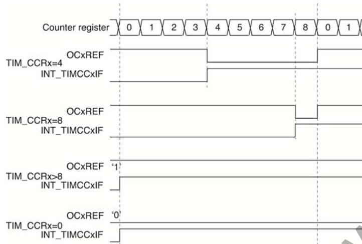
**Figure 9.22. Edge-Aligned PWM Waveforms (ARR = 8)**
