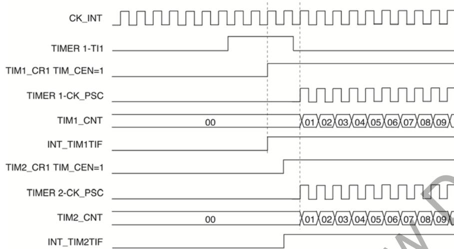
**Figure 9.36. Triggering Timer 1 and 2 with Timer 1 TI1 Input**
