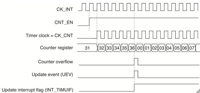
**Figure 9.3. Counter Timing Diagram, Internal Clock Divided by 1**
