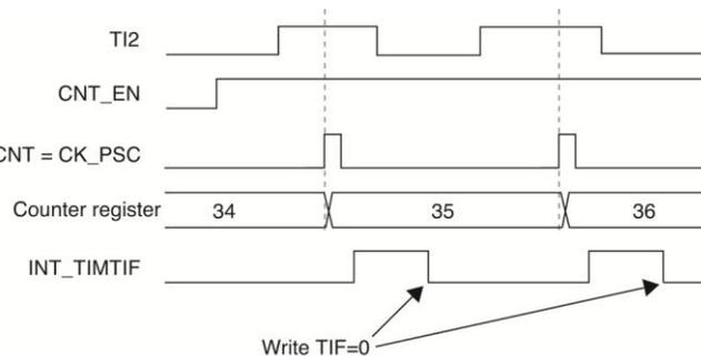
**Figure 9.14. Control Circuit in External Clock Mode 1**
