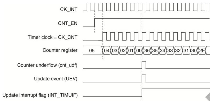
**Figure 9.7. Counter Timing Diagram, Internal Clock Divided by 1**
