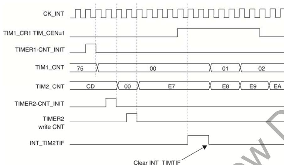
**Figure 9.35. Triggering Timer 2 with Enable of Timer 1**
