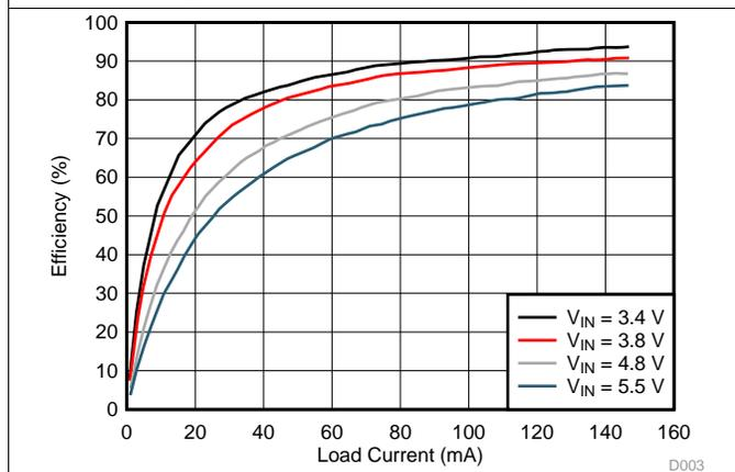
Figure 4. Forced PWM Efficiency vs Output Current
