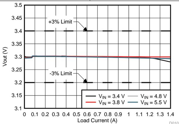
Figure 16. Load Regulation vs Output Current
