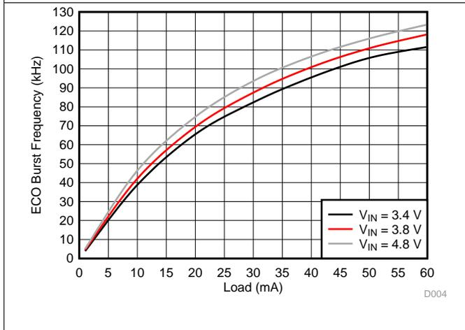
**Figure 10. ECO Burst Frequency vs Output Current**
