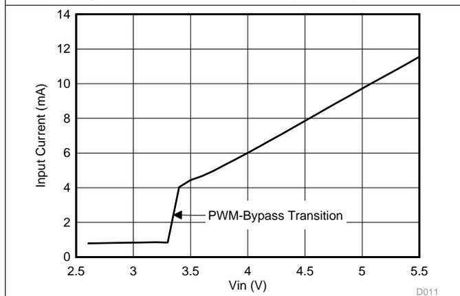
Figure 6. No Load Forced PWM Input Current vs  $V_{IN}$
