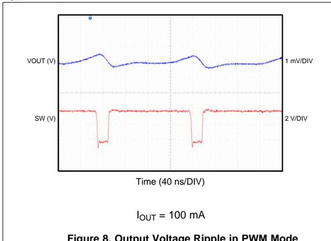
**Figure 8. Output Voltage Ripple in PWM Mode**
