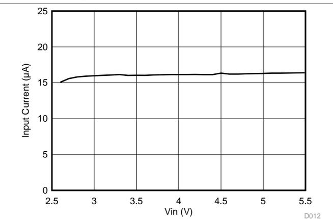
Figure 5. No Load ECO Input Current vs  $V_{IN}$
