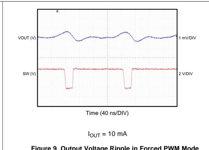
**Figure 9. Output Voltage Ripple in Forced PWM Mode**
