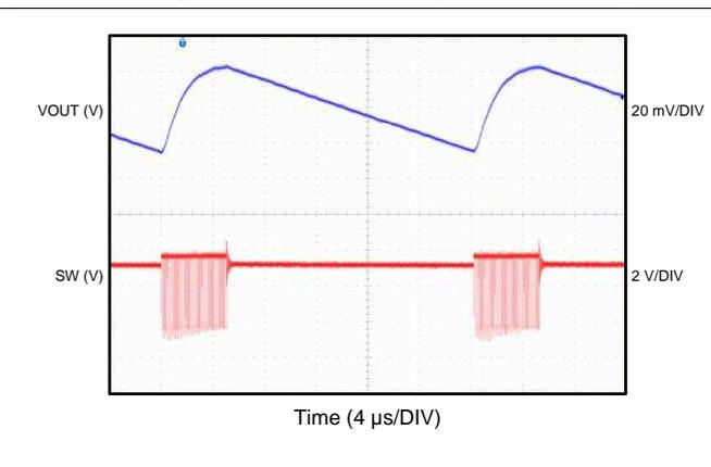
Figure 7. Output Voltage Ripple in ECO Mode
