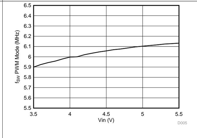
**Figure 11. PWM Switching Frequency vs  $V_{IN}$**
