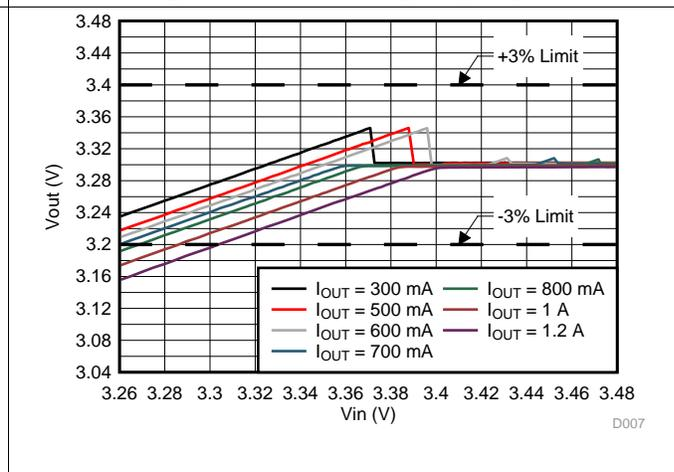
**Figure 13. Analog Bypass-to-PWM Transition, Rising  $V_{IN}$**
