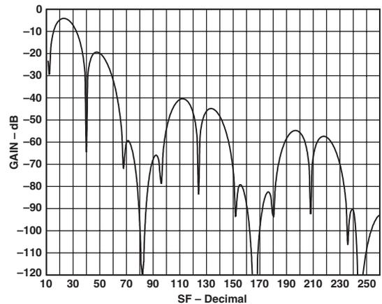
Figure 13. 50 Hz Normal Mode Rejection vs. SF
