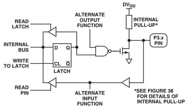
Figure 41. Port 3 Bit Latch and I/O Buffer
