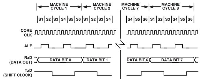
*Figure 54. UART Serial Port Transmission, Mode 0*
