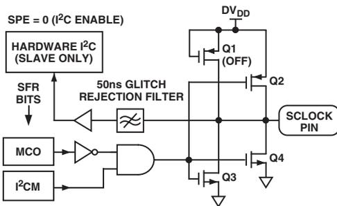
Figure 43. SCLOCK Pin I/O Functional Equivalent in I<sup>2</sup>C Mode
