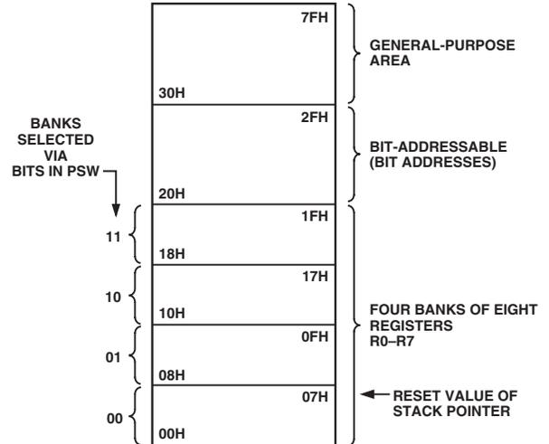
Figure 2. Lower 128 Bytes of Internal Data Memory
