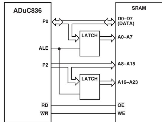
Figure 60. External Data Memory Interface (16 Mbytes Address Space)
