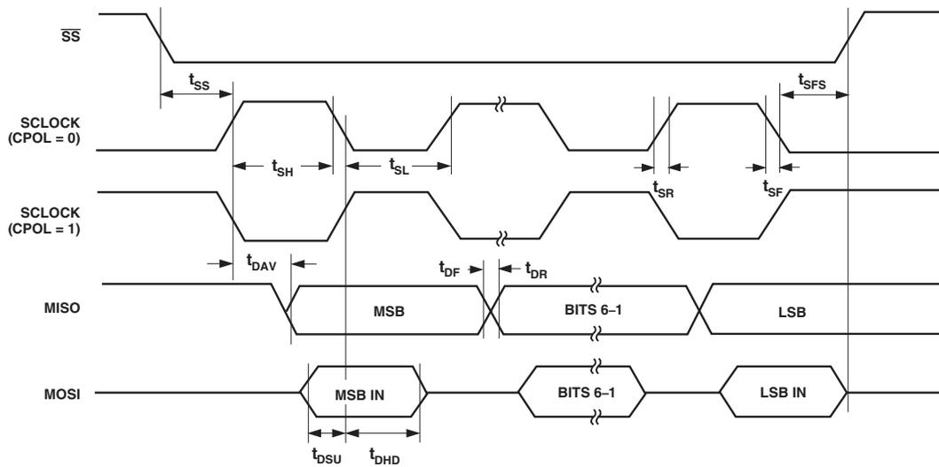
Figure 77. SPI Slave Mode Timing (CPHA = 1)
