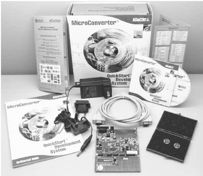
Figure 67. Components of the QuickStart Development System
