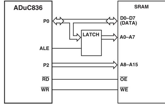
Figure 59. External Data Memory Interface (64 Kbytes Address Space)
