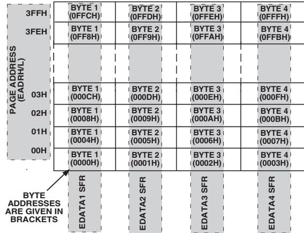
Figure 20. Flash/EE Data Memory Control and Configuration
