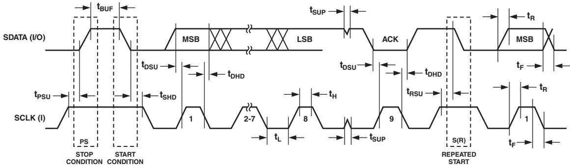
Figure 79. I<sup>2</sup>C Compatible Interface Timing
