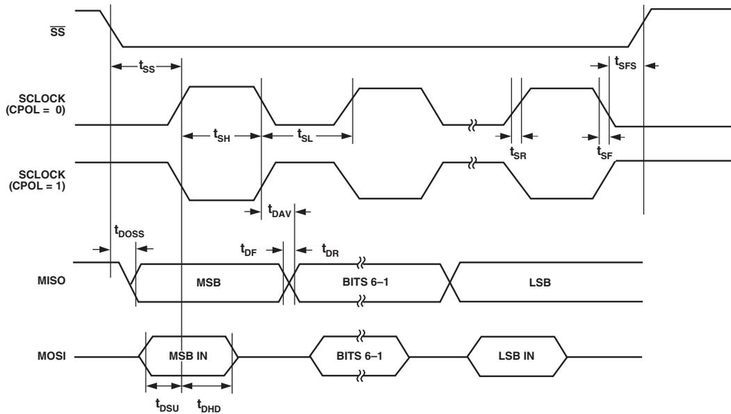
Figure 78. SPI Slave Mode Timing (CPHA = 0)
