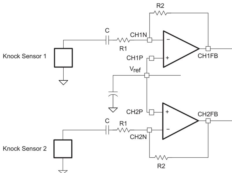
NOTE: The series capacitor C is not mandatory and may be removed in some application circuits
