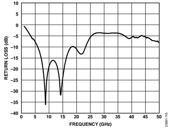
Figure 15. Return Loss vs. Frequency at  $V_{TUNE} = 6 V$
