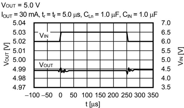
(2) Transient Response Characteristics of Load (Ta = 25°C)
