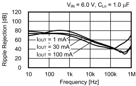
**Remark** C<sub>Ln</sub>: Capacitor set to VOUTn pin externally (n = 1, 2)
