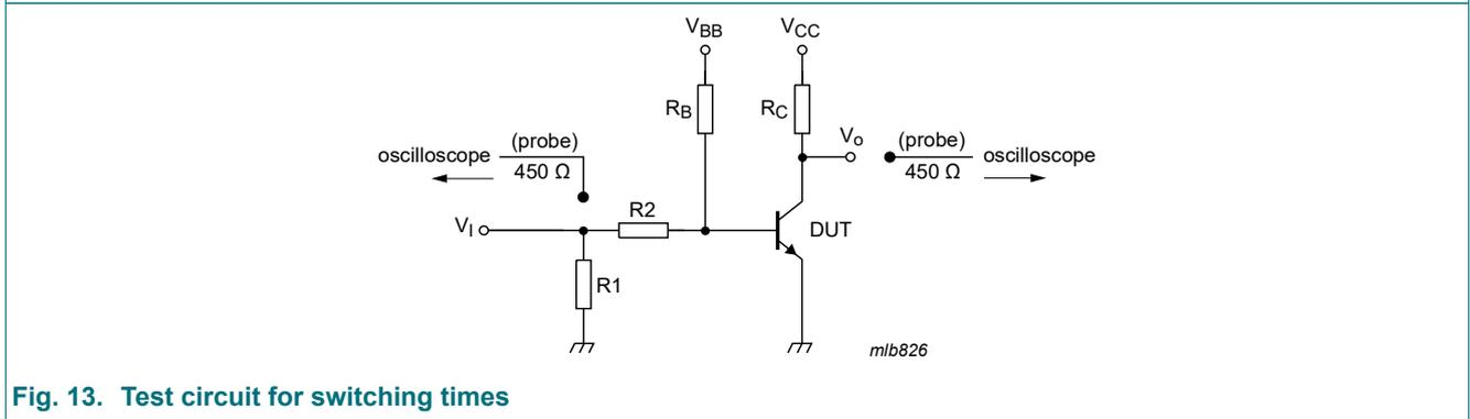
Fig. 13. Test circuit for switching times
