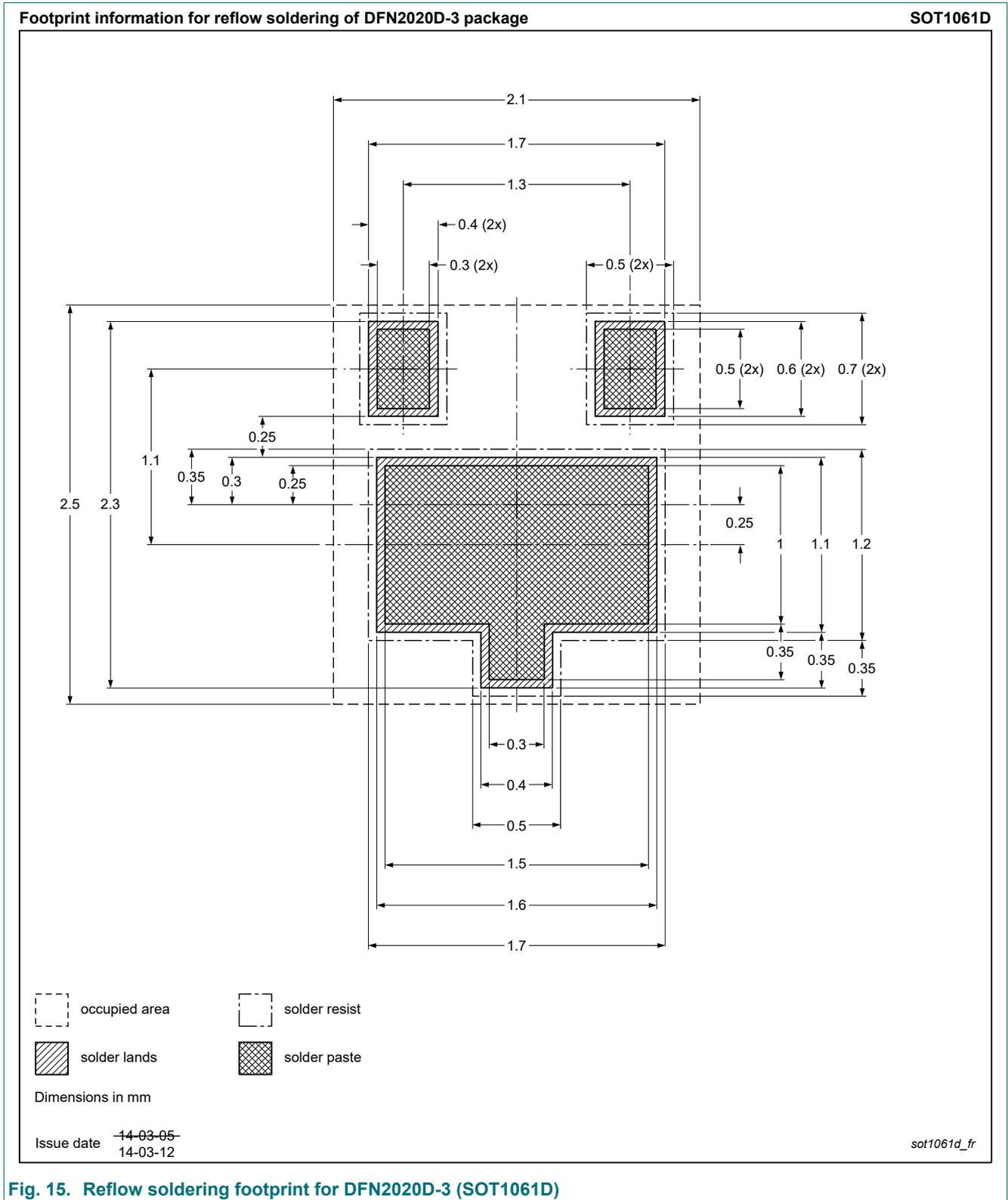
Fig. 15. Reflow soldering footprint for DFN2020D-3 (SOT1061D)
