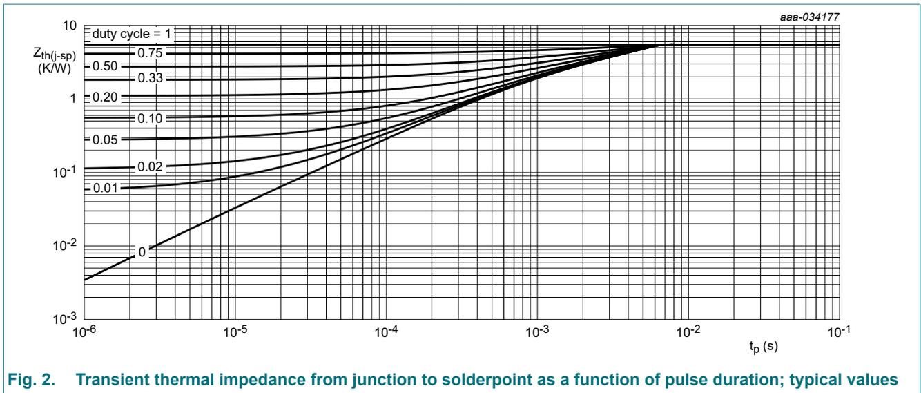
Fig. 2. Transient thermal impedance from junction to solderpoint as a function of pulse duration; typical values
