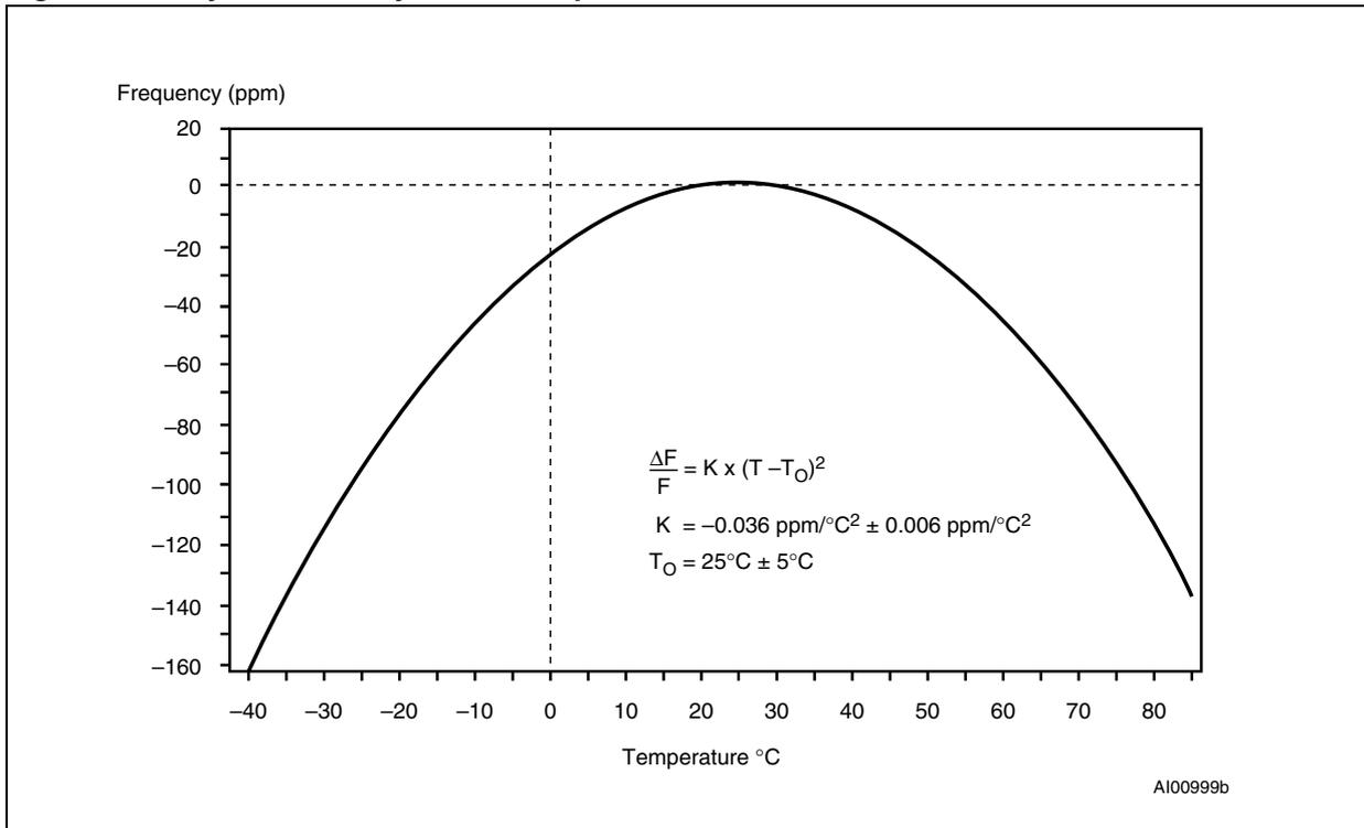
Figure 13. Clock calibration
