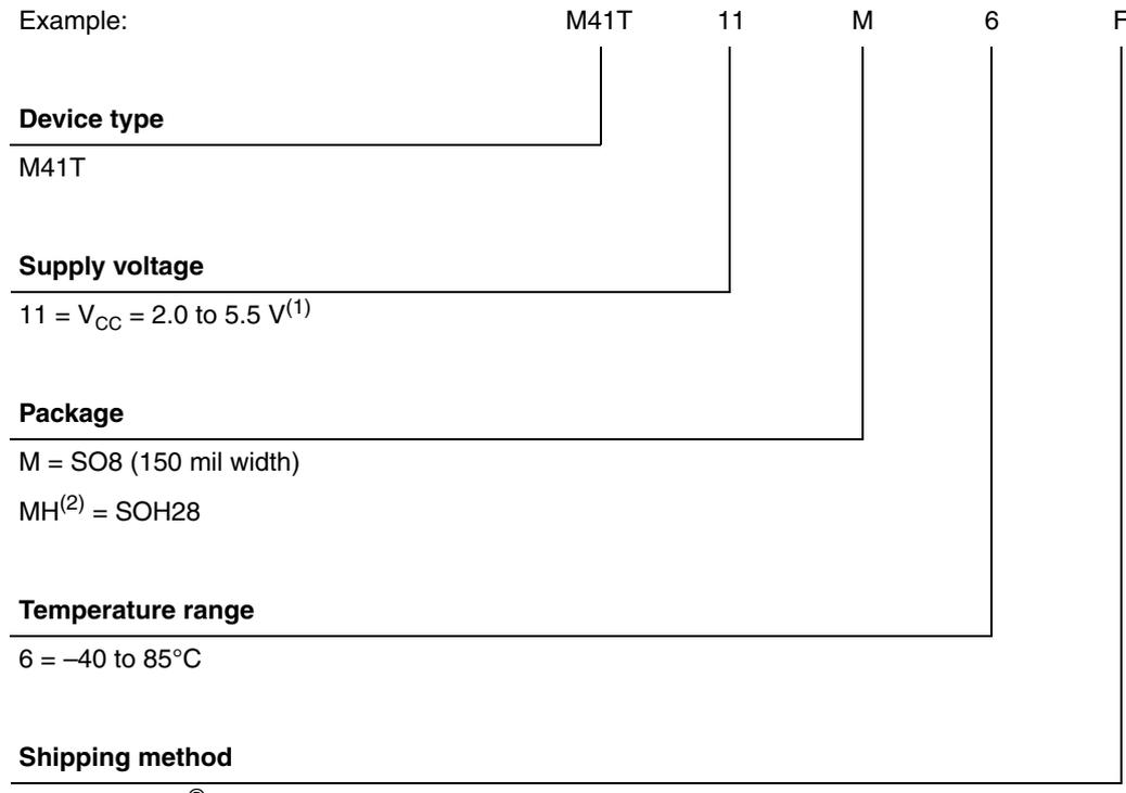
1. SOH28 supply voltage is 3.3 V to 5.5 V.
