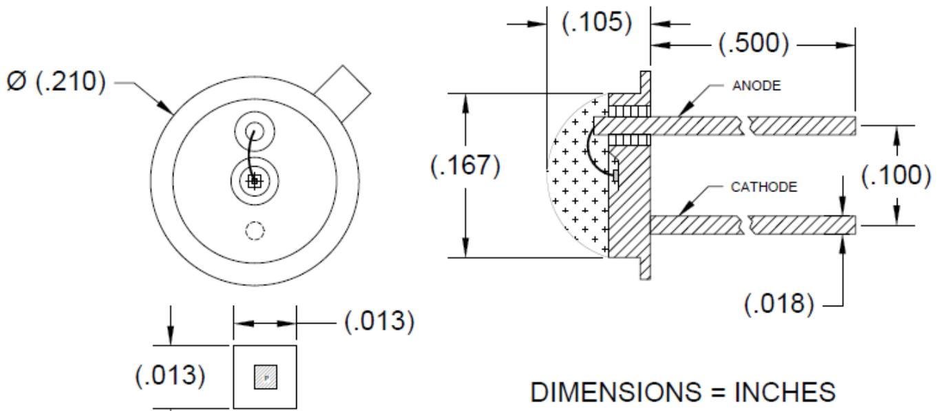
>Soldering Conditions: 260°C 1/16 inch away from case for 3 seconds max.
