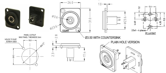
CP303100 - XRP3 with 3.5mm Vertical Stereo Jack Socket - PC Mounting, CSK Hole CP303100X - XRP3 with 3.5mm Vertical Stereo Jack Socket - PC Mounting, Plain Hole
