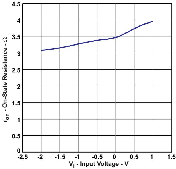
Figure 1. ON Resistance vs V<sub>1</sub> for Audio Switch
