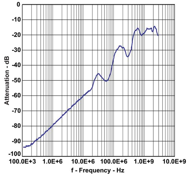
Figure 8. Cross Talk vs Frequency for USB Switch
