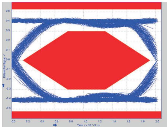
Figure 9. USB 2.0 Eye Pattern for USB Switch
