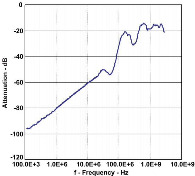
Figure 7. Cross Talk vs Frequency for Audio Switch
