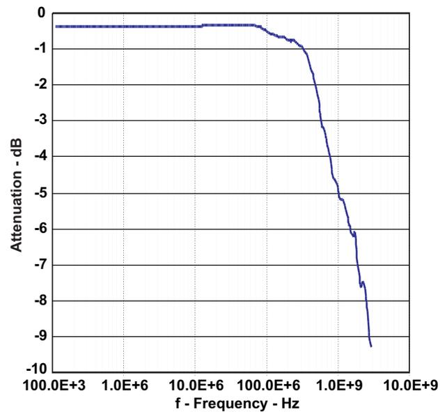
Figure 4. Gain vs Frequency for USB Switch
