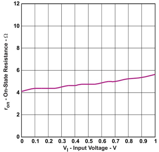
Figure 2. ON Resistance vs V<sub>1</sub> for USB Switch
