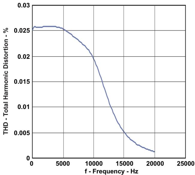
Figure 3. THD vs Frequency for Audio Switch
