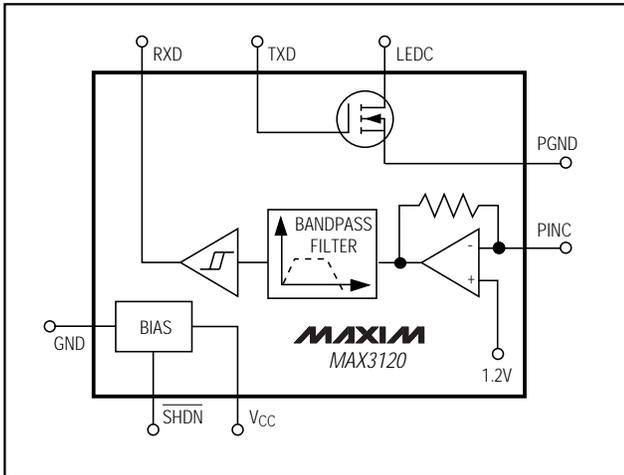
Figure 1. Functional Diagram
