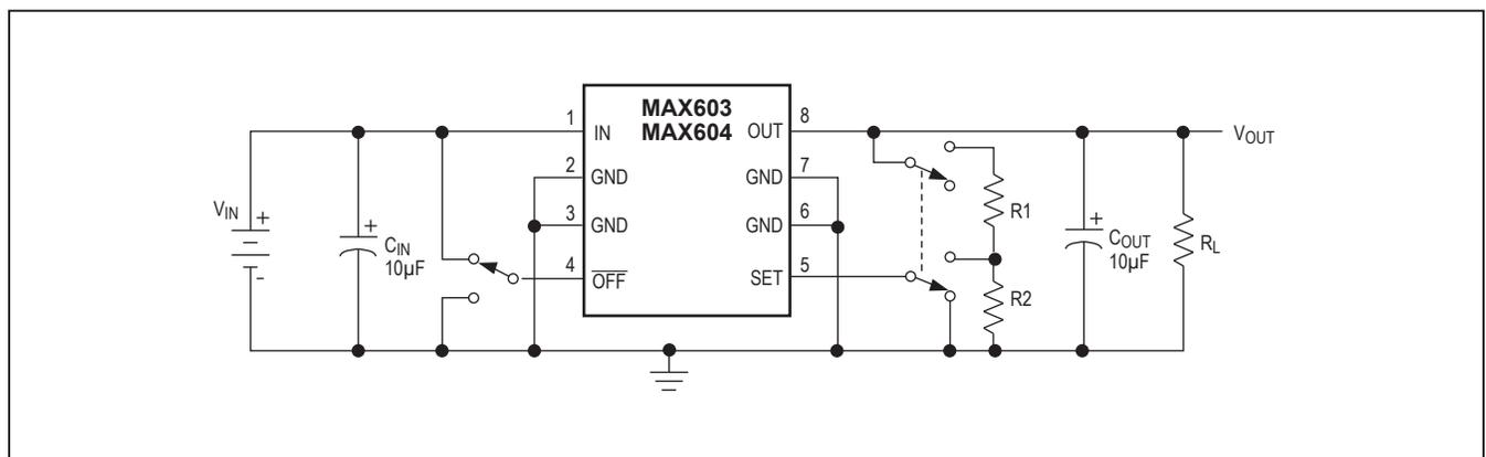
Figure 1. Test Circuit
