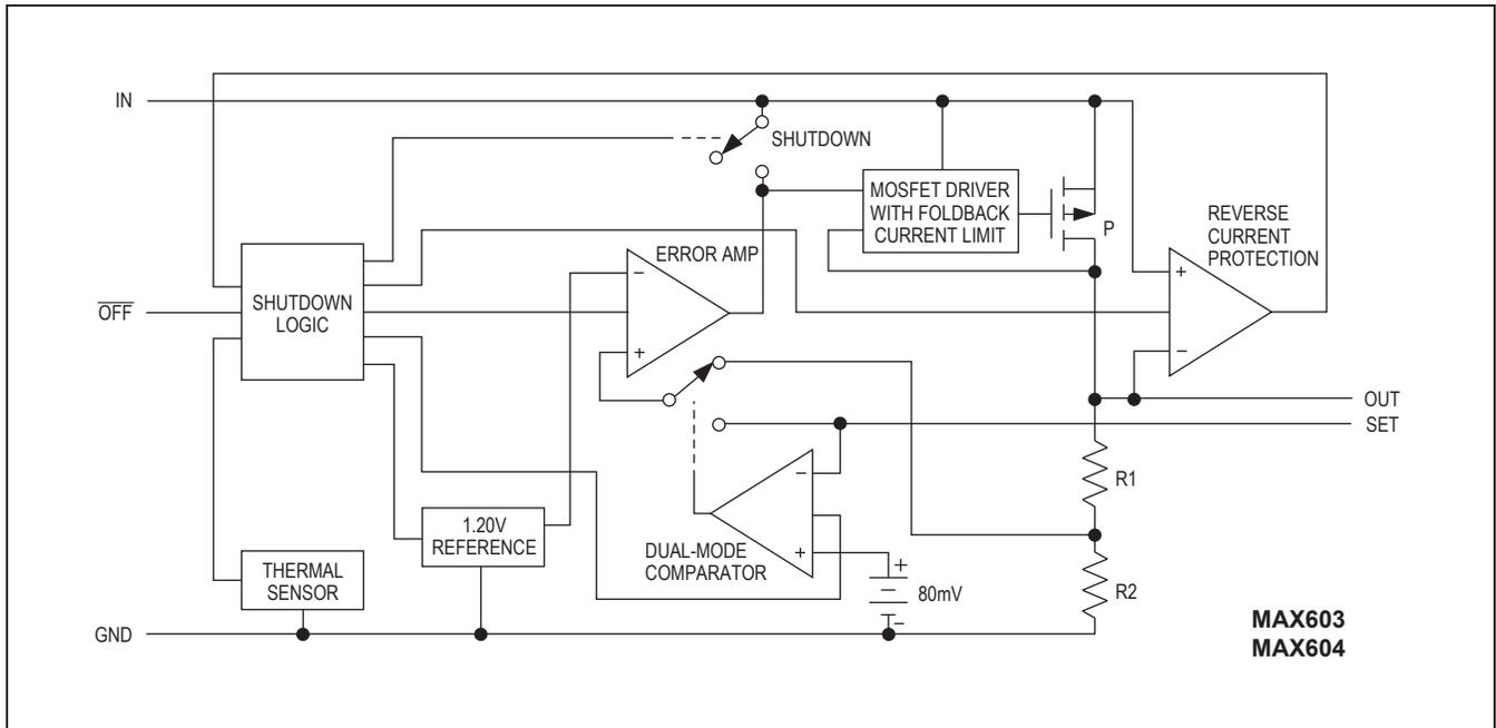
Figure 2. Functional Diagram
