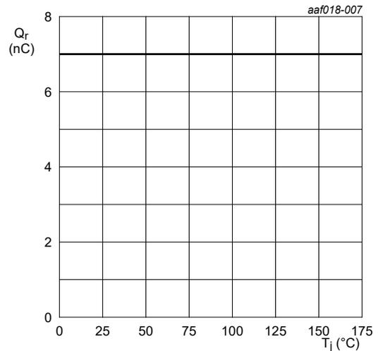
**Fig. 7. Recovered charge as a function of junction temperature**
