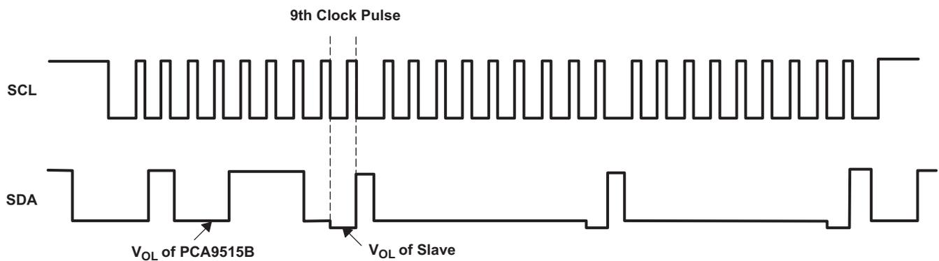
Figure 7. Bus 1 Waveforms
