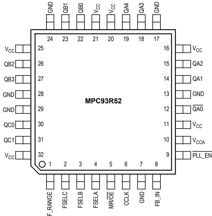
It is recommended to use an external RC filter for the analog power supply pin V<sub>CCA</sub>. Please see application section for details.
