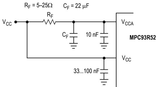
Figure 7.  $V_{CCA}$  Power Supply Filter
