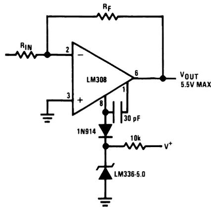
Figure 18. Bipolar Output Reference
